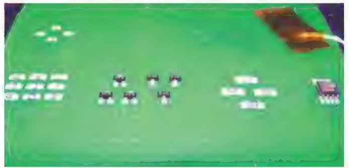
Figure 17. Board placed in oven with thermal sensor attached.
